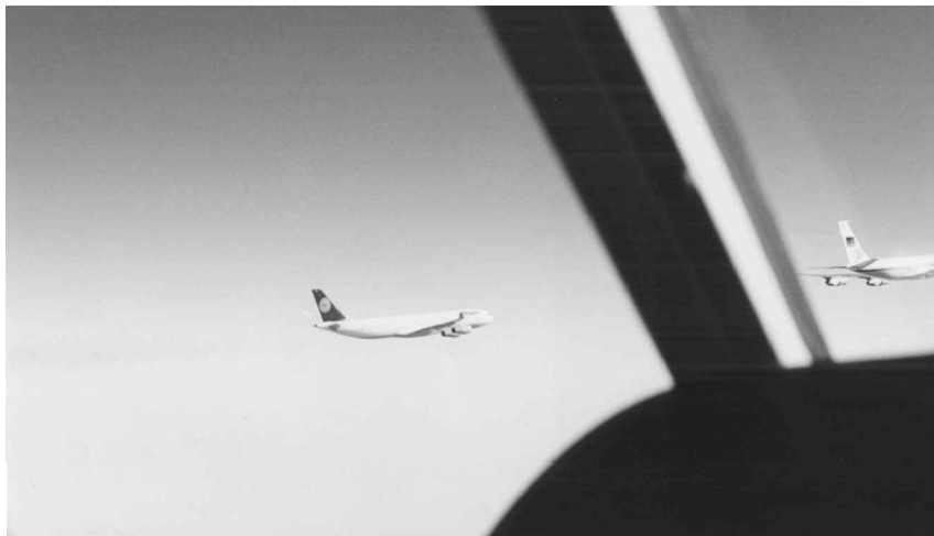
Fig. 2 Airbus A340 with contrails (left) and the Boeing B707 without contrails (right) taken from the Falcon research aircraft at about flight level 333 hft at 7:28 UTC, 15 Sept. 1999 (photographs: U. Schumann and R. Welsler, DLR).
